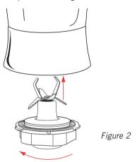
**Note:** The blender jug will leak if the sixblade system is not assembled correctly.
