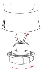
Remove the rubber seal from the blade assembly. Wash the blender lid, ingredient cup, rubber seal, blade assembly and blender jug in warm soapy water.
