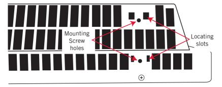
Positioning is only possible in the one orientation, either foot can be used at either end.
