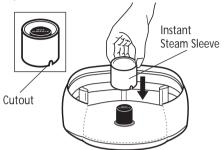
The Sleeve concentrates a small amount of water around the Exposed Heating Element, quickly bringing it to boiling temperature to produce steam, rather than heating all of the water in the reservoir.
