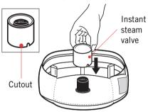
The Sleeve concentrates a small amount of water around the Exposed Heating Element, quickly bringing it to boiling temperature to produce steam, rather than heating all of the water in the reservoir.
