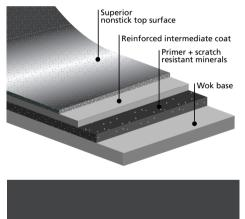
Teflon Platinum is a premium 3 layer nonstick coating. It features special scratch resistant minerals causing metal utensils to slide over these particles without damaging the Teflon matrix.
