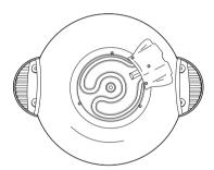
Completely cast-in element
