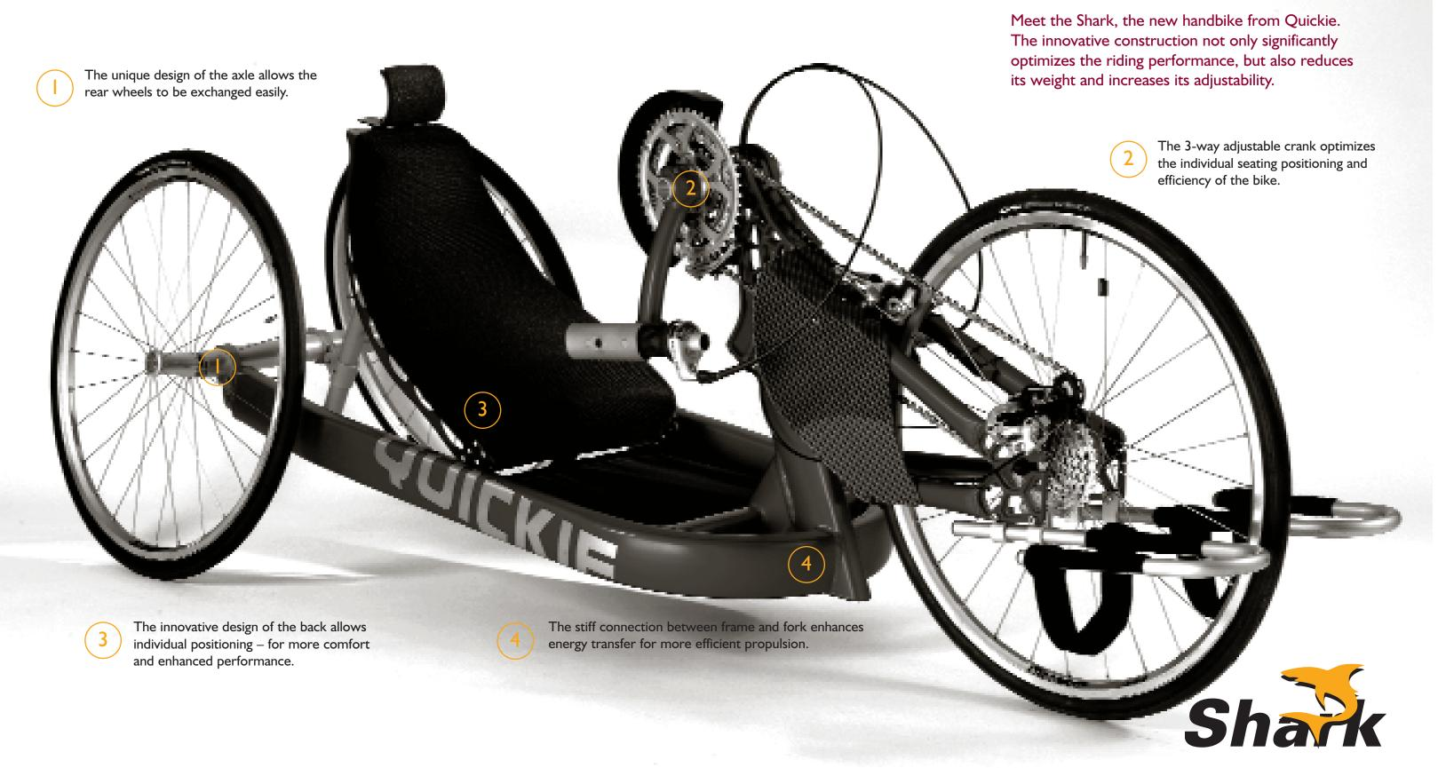
The features, which optimize the efficiency of the bike in competitions, also enhance comfort and performance in leisure time, such as the adjustable crank, the adjustable back and the reduced weight. The Shark can also be folded and comes with a special support which is fixed to the frame. This makes the transport and the handling of the bike extremely easy.
