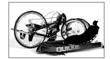
The special support allows the bike to be set up in a stable position. The fork is easily removed, and the rider can comfortably get off the handbike.
