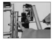
b. Remove the two block bolts with a phillips screwdriver and a 7/16" socket wrench.
