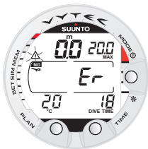
Fig. 3.32. Surface Mode after a violated decompression dive. Er symbol indicates that you have violated the ceiling for more than three minutes. You must not dive again for at least 48 hours.
