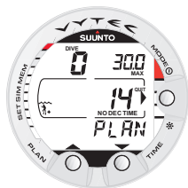
Fig. 3.6. Dive Planning. Planning mode is indicated by PLAN text. No-decompression time limit at 30.0 m [100 ft] is 14 minutes in A0/P1 mode.
