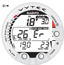
Fig. 3.19. Decompression dive, above ceiling. Note downward pointing arrow, Er warning and an audible alarm. You should immediately (within 3 minutes) descend to or below ceiling.
