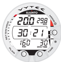
Fig. 3.28. Diving in Gauge mode. Current dive time is 30 minutes 21 seconds.
