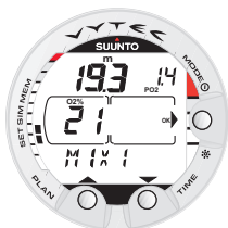
Fig. 3.27 Changing gas mix. Current gas mix is MIX1 (21%). Scroll through enabled mixes by pressing PLAN or TIME button. Select new mix by pressing MODE (OK) button.
