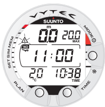
Fig. 3.31. Surface interval, no-flying time. Pressing TIME button twice will show no-flying time, indicated by an airplane symbol.
