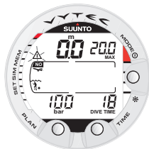
Fig. 3.29. Surface display. You have surfaced from a 18 minute dive, which maximum depth was 20.0 m [66 ft]. The present depth is 0.0 m [0 ft]. Airplane symbol indicates that you should not fly and blinking Diver Attention Symbol indicates that you should prolong your surface interval time because of excess micro-bubbles.
