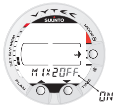
Fig. 4.29. Setting additional gas mixes (MIX2, MIX3). MIX 2 is turned off. Press scroll buttons to enable/disable MIX2. Press MODE (OK) to accept settings.
