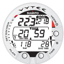
Fig. 3.15b Deepstop. Arrows indicate you are at the deep stop depth. There is 59 seconds left to complete the deepstop.
