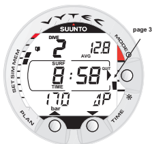
Fig. 4.9. Logbook, page III. Surface interval time, average depth and consumed air indicated by \Delta P .
