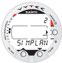
Fig. 4.19. Dive Planning Simulator mode. [2 SIMPLAN].
