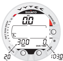
Fig 3.3. Startup III. Surface mode. Depth and dive time are zero and cylinder pressure is 300 bar [4350 psi]. Pressing TIME button activates alternative display of temperature and current time.
