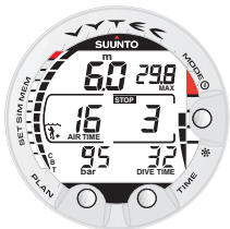
Fig. 3.11. A three minute Recommended Safety Stop.
