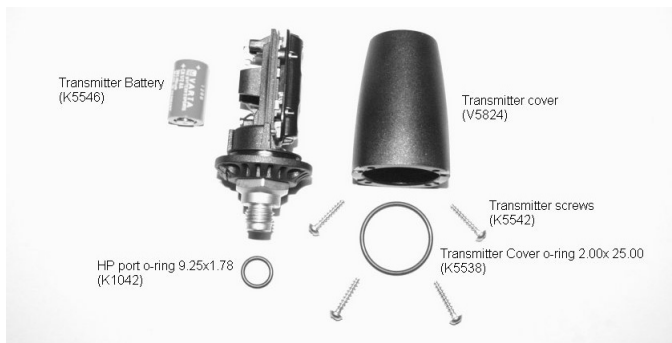
Fig. 5.3 Wireless transmitter parts. The code stands for spare part order number.
