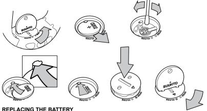
Make sure that you have purchased an original Suunto battery kit (including battery and battery lid with installed O-ring) before you start replacing the battery.
