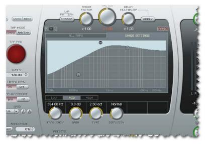
The Shade settings basically define a 3-band parametric EQ that is applied to all delay taps.
