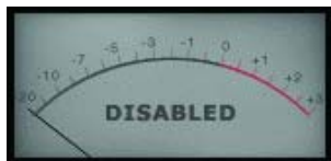
Figure 2: The 24/7•C will appear as though the "lights are out" and the disabled message will appear in the VU Meter display.
