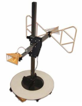
The TDK DAPS-01 Dual Antenna Positioning System is designed to simply testing by enabling remote positioning of two antennas in EMC test environments.
