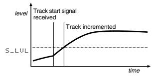
A fall and subsequent rise in volume alone when recording digitally from CD, MD or DAT is not sufficient to trigger an automatic track increment.
