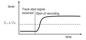
• when recording digitally from a CD or MD deck, a digital track start signal is received, and the signal level subsequently rises above the trigger level:
