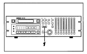
¶ Simply press LOC 1 to have the DA-38 autolocate to the location currently stored into the MEMO 1 register, or press LOC 2 to have the unit autolocate to the current MEMO 2 location.
