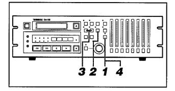
When you rotate the SHUTTLE knob for reel rocking to locate specific points on the tape, what you hear depends on whether the shuttle monitor mode is activated or not, as shown in the table below.
