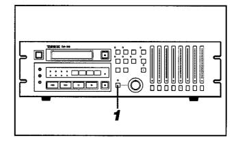
Press the SHUTTLE switch and the associated LED will light.
