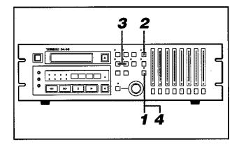
1 Press the SHIFT key and the associated LED will start blinking to show that all the double function keys are switched to offer their lower blue-labelled functions.
