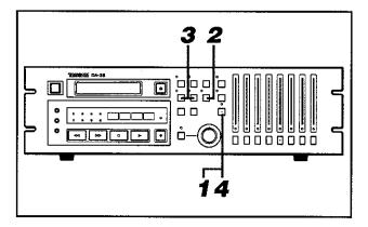
1 Press SHIFT and the associated LED will start blinking to show that all the double function keys are switched to offer their lower blue-labelled functions.
