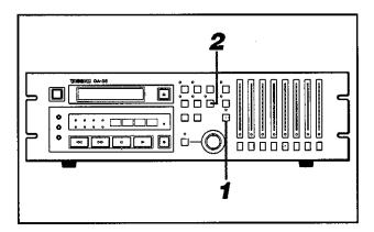
Press SHIFT and the associated LED will start blinking to show that all the double functions keys are switched to offer their lower blue-labelled functions.
