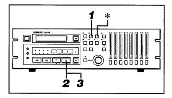
1 Press the AUTO IN/OUT key and the associated LED will start blinking to show that the unit is in Auto punch-in/out ready mode.
