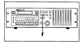
This causes the inputs whose corresponding tracks are record enabled to be sent directly to the same numbered outputs whenever the transport goes into any other modes than play.
