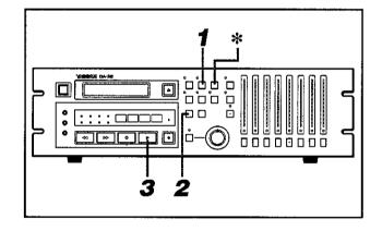
¶ Press AUTO IN/OUT and the associated LED will start blinking to show that the unit is in Auto punchin/out mode.
