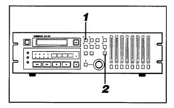
1 Check to see that the RHSL LED is lit. If it isn't, press the RHSL key two times and the LED will light.
