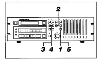
Press SHIFT and the associated LED will start blinking to show that all the double function keys are switched to offer their lower blue-labelled functions.
