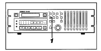
ALL INPUT is used to switch the eight outputs to be fed directly by the corresponding inputs.
