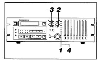
1 Press SHIFT and the associated LED will start blinking to show that all the double function keys are switched to offer their lower blue-labelled functions.
