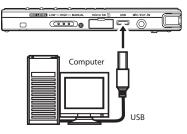
When connected to a computer, a pop-up window appears on this unit's display to let you choose whether you want to operate the unit using USB bus power or to connect the unit with the computer by USB.
