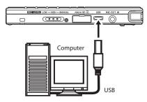
If you connect the unit by USB when its power is ON, or if you turn the unit's power ON when it is already connected by USB, a screen appears on this unit's display to let you choose whether you want to operate the unit using USB bus power or to connect the unit with the computer by USB.
