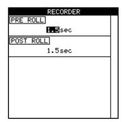
There are only two parameters here, used to change the pre-roll and post-roll times of the auto punch operation (see "Auto punch operations" on page 55).
