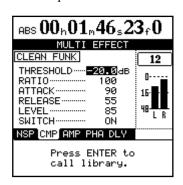
At the bottom of the screen, each of the effects in the multi-effect is shown with an abbreviation. These effects are connected in a chain in the order displayed. This order cannot be changed.
