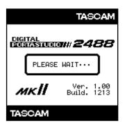
After about 20 seconds, the 2488MKII will be ready and the HD (hard disk) indicator stops flashing. Adjust the display so that it is comfortable for you to read, using the contrast control.
