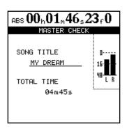
All monitoring is now from the STEREO selection only. The master track playback sound is not affected by fader movements or other mixer operations, including new assignments.
