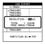
6 Select the final bit depth (RESOLUTION) of the exported files (16 or 24 bits). The file size of the exported data changes according to the bit depth.
