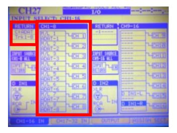
The output page must also be setup to send DIRECT 1-8 to the ADAT output.
