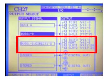
To record in Pro Tools from the DM-24, you must assign your Pro Tools tracks to receive their input from the ADAT connection sent from the DM-24 direct outputs.
