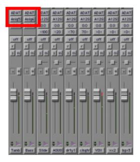
In the example below, channels 17-32 are setup to receive 14 tracks from the 001 - 8 tracks via ADAT digital I/O and 6 tracks from the analog I/O. These channels are all assigned to the stereo buss of the DM-24.
