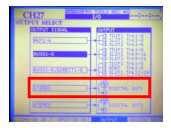
In Pro Tools, create a stereo aux input. Set the input to S/PDIF. This is where the stereo buss signal of the DM-24 is sent to Pro Tools. This signal is assigned to the Pro Tools stereo buss.
