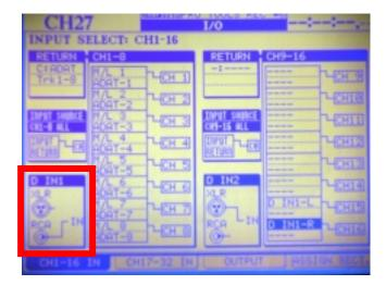
On the DM-24 DIGITAL-CLOCK page, set the DM-24 to clock to the D-1 IN (RCA.)
