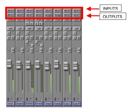
You must also assign your outputs. This is where you decide what tracks you want to mix in the DM-24, and what tracks you want to mix in Pro Tools. In the example below the Tambourine is sent to analog output 5, the Bass is being sent to analog output 6 and the other tracks are being sent to the Pro Tools stereo buss.
