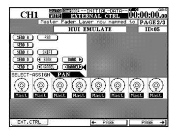
SEND A-E refer to aux sends. If you point to A and press ENTER, the encoders on the LCD will show you all of the levels for the first aux send on the channels viewed. Using the cursors, you can highlight the encoder area and adjust them 4 at a time.
