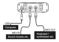
You can use the MIDI IN/MIDI OUT connectors to transmit and receive MTC (MIDI Time Code). This allows the MTC-compatible DAW (Digital Audio Workstation) computer application to synchronize with your MIDI equipment.
