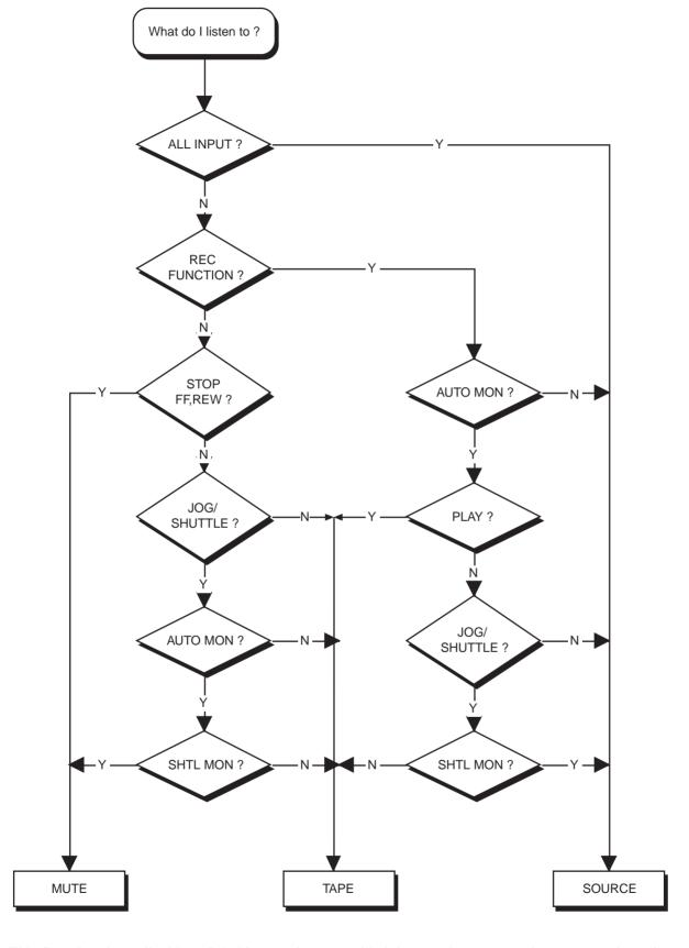
This flowchart is applicable to DA-98 operations, provided that you have not made any manual monitor settings using the **INPUT MONITOR** keys, and that confidence mode is off.
