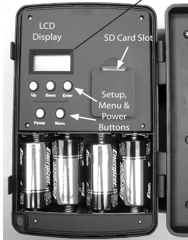
Control Panel (Front Opened)
