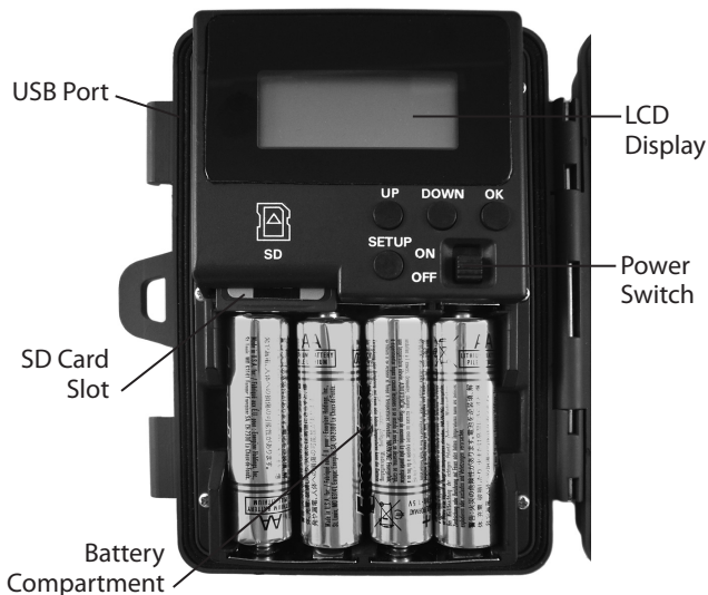
Control Panel (Front Opened)
