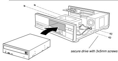
**4c**) Locate the secondary IDE connector on your system's motherboard and connect one end of the IDE interface cable.
