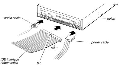
**4e**) Connect one end of an analog audio cable to the analog audio connector on the rear panel of the CD-RW drive and connect the opposite end to your sound card. **(Go to Step 6.)**
