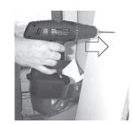
Make sure that the driver bit is inserted straight in the screw head or the screw may become damaged or will not be inserted properly. When driving wood
