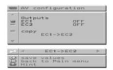
Once the copy direction has been set (e.g. EC1 → EC2), the outputs of the appropriate SCART sockets will switch to OFF. If EC1 or EC2 are set to OFF, this means that no TV output signals will be directed to the SCART socket.
