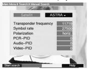
This menu differs from the **Transponder** nmenu only in terms of the menu points **PCR-PID**, **Audio-PID** and **Video-PID**.
