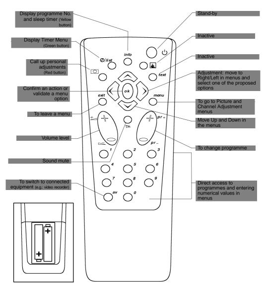
**Batteries:** Remove the lid at the back of the remote control and insert two 1.5 V, LR06 batteries.
