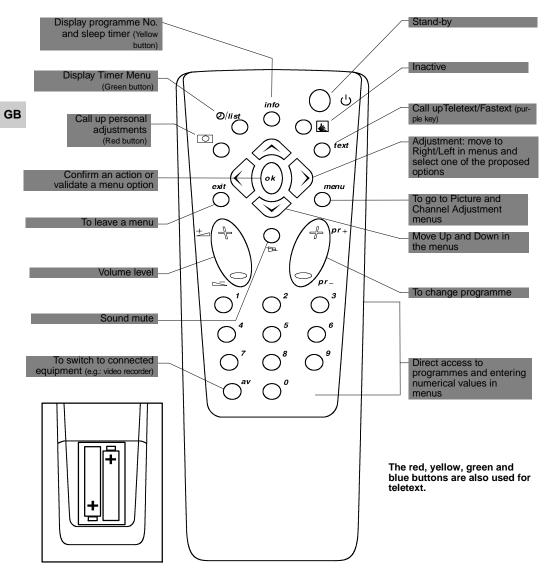
**Batteries:** Remove the lid at the back of the remote control and insert two 1.5 V, LR06 (AA) batteries.
