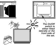
The TV set has been designed for use in dry rooms. Should you exceptionally operate it in the open air (example: on the balcony, in the veranda or tent), you must absolutely protect it against moisture (dew, rain, splash water). Prior to put up into operation a cold TV set in a warm room, you should wait until the possibly misted-up screen has dried by itself. In no case should you dismantle your TV set yourself.
