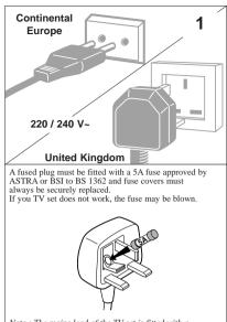
Note: The mains lead of the TV set is fitted with a moulded plug. Because it contains safety components we cannot recommend re-wiring.
