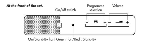
Press the on/off switch; the indicator light comes on.
