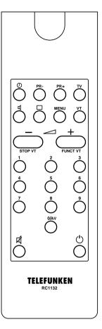
Batteries : Remove the lid at the back of the remote control and insert two 1,5 V batteries, TYPE LRO3 (AAA) or equivalent.
