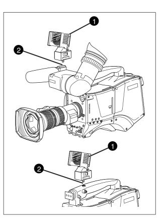
To mount a top light ① onto the camera, proceed as follows:
