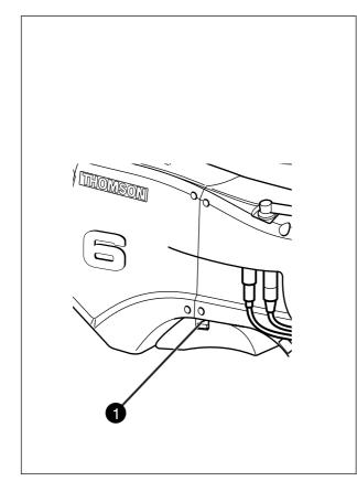
To change the position the shoulder pad press and hold lever ①. The shoulder pad can now be moved backwards and forwards along the axis of the camera. Adjust the shoulder pad when all units have been mounted so that the best balanced position can be obtained.
