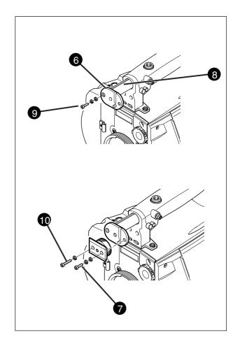
When wearing headphones it may be necessary to move the viewfinder further to the left to obtain a more comfortable viewing position. A right eye adapter **(3)** is supplied for this purpose. Mount the right eye adapter as follows:
