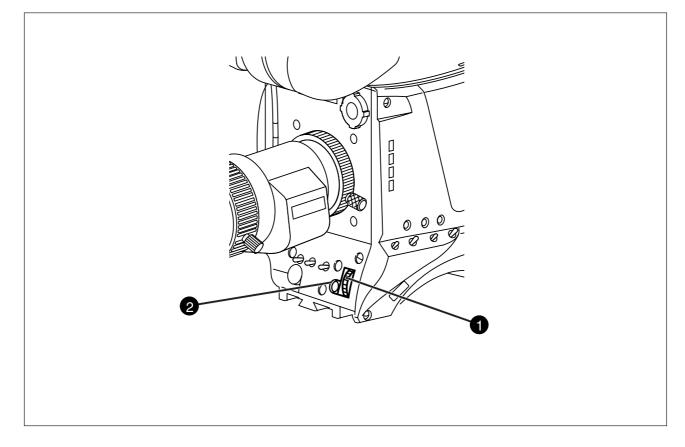
The system menus are displayed in the viewfinder. There are two controls at the front of the camera that allow you to navigate through these menus.
