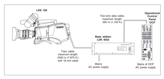
In this mode the camera is connected to a base station via a Triax adapter and cable. Remote control of the camera is achieved by a remote control panel of the Series 9000 Control System. This can be an operational control panel (OCP) connected to the base station. The data communication between camera and base station is carried over the Triax cable. **Section 4**
