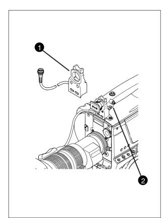
An optional zoom control unit ① can be mounted on the carrying handle. The three available versions for different types of lens are:
