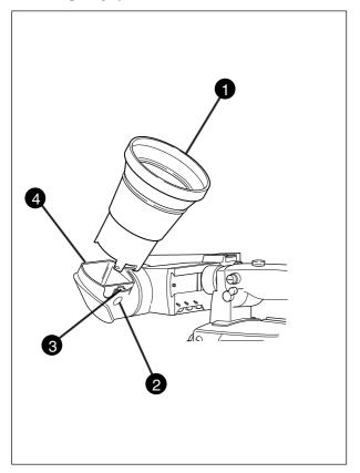
If you regularly use the viewfinder at a distance, for example, when you use the camera in the hand-held position, it is recommended that you fit the optionally available wide angle eyepiece (LDK 5390/00).
