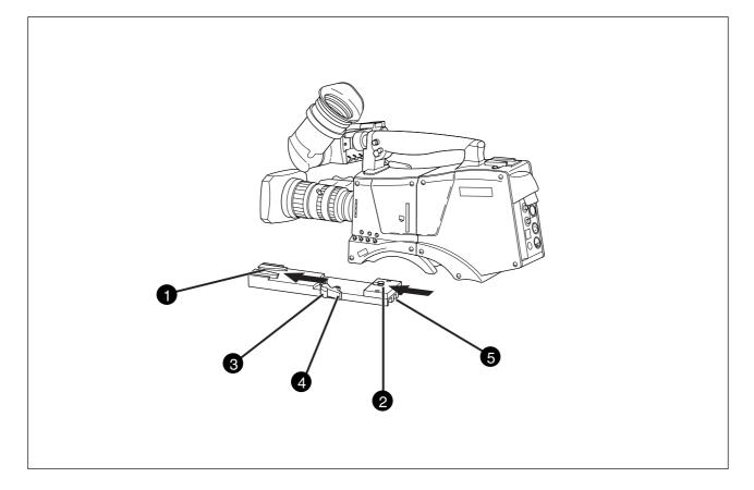
To mount the camera on a tripod, the tripod plate (LDK 5030/00 is delivered as standard) must first be attached to the tripod.
