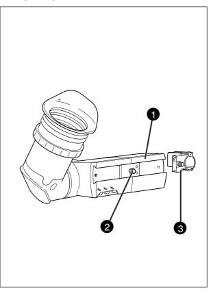
A left eye adapter is optionally available (LDK 5390/10) to allow the viewfinder to be used with the left eye.
