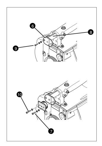
When wearing headphones it may be necessary to move the viewfinder further to the left to obtain a more comfortable viewing position. A right eye adapter is supplied for this purpose. Mount the right eye adapter as follows:
