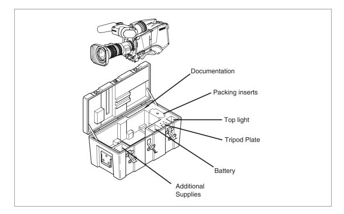
It is important to protect your camera against damage when transporting it. To do this, a transport case (LDK 5020/00) is optionally available for the camera, lens, viewfinder and some accessories.
