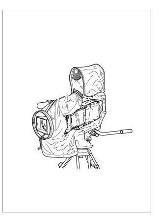
The rain and off-use cover must be used when the camera system is in a wet or damp environment. This protection is necessary for personal safety reasons. The cover can also be used indoors to protect the camera when it is used in dusty environments. It can also be useful if the camera is being put into storage. For more information on how to put on the cover refer to the User's Guide which is supplied with it.
