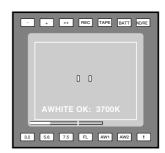
The measured colour temperature is now stored in the selected memory position and can be recalled as required. The camera is now ready for use.
