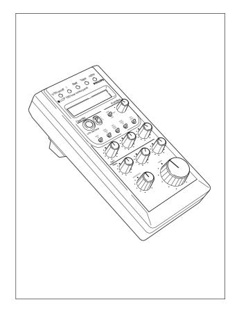
The optional Local Control Panel, the LCP100 for the LDK 100 series (LDK5201/00), allows the operator to control the camera remotely. The LCP 100 controls the Iris, the Master Black, and black and white painting. The LCP 100 menu is used to access the major camera settings. The LCP 100 menu settings and the associated values are displayed on the 16 character LCD.
