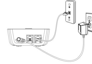
2. Plug one end of the telephone line cord in the LINE IN jack on the back of the base and the other end into a modular jack.
