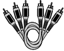
RCA sockets and cables for Y, Pr, Pb Video signals, also called Component.
