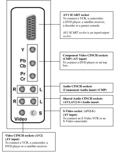
To display images from the connected appliance, select the input source by pressing the AV button on the remote control (see page 13).
