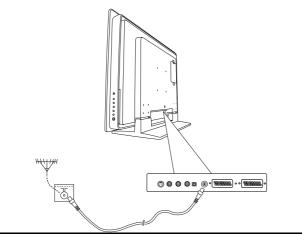
**3.** Connect the outside aerial or cable network to the socket at the back of the TV set.
