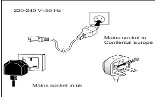
Equipment for the UK is supplied with a mains cable fitted with a moulded plug.
