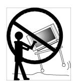
**22.Panel protection**—The LCD panel used in this product is made of glass. Therefore, it can break when the product is dropped or impacted upon by other objects. Be careful not to be injured by broken glass pieces in case the LCD panel breaks. Include
