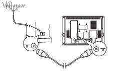
Connect the outside aerial or cable network to the ¬r socket at the back of the TV set.
