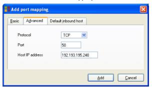
By default, the IP address of the PC from which you are running the NAPT Manager will be taken as host IP address. To add a NAPT entry for another PC, you must change the proposed IP address.
