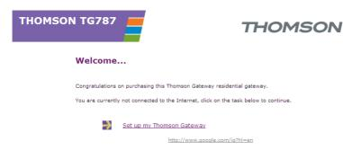
If this window does not appear browse to <a href="http://dsldevice.lan">http://dsldevice.lan</a> or to the IP address of your Thomson Gateway (by default: <a href="https://dsldevice.lan">192.168.1.254</a>) and click **Thomson Gateway** on the menu on the left-hand side.
