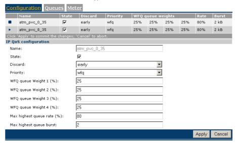
Quality of Service allows specifying a connection service guarantee via a set of connection parameters. Throughout the network, this set of connection parameters will be used to handle the connection data in a way to achieve the connection service guarantee. This handling includes reserving bandwidth, priority based queuing, scheduling, modifying data characteristics, ...
