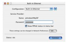
Make sure Built-in Ethernet is selected in the Configuration list.
