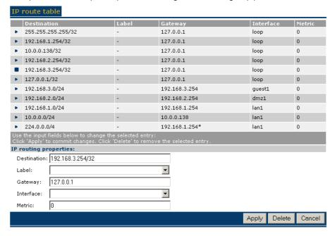
Similar to the IP address table, a number of IP Routes are pre-configured. Other routes are either added via adding an IP address manually, or via the address negotiation of a Packet Service connection session, e.g. for Routed PPPoA's or Routed PPPoE's IPCP, via the DHCP client, e.g. for Routed Ethernet (MER), via pre-configuration, for example for Routed IPoA, or by the Routing Information Protocol.
