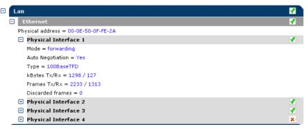
The LAN Diagnostics provide information on the SpeedTouch™'s local network Ethernet interface(s).
