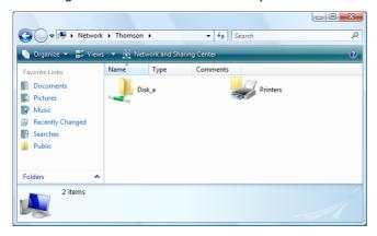
If the storage device has multiple partitions an index number will be added at the end (for example: Disk\_a1 and Disk\_a2).
