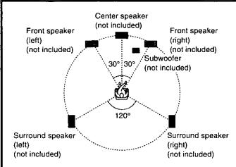
The front, center, and surround speakers should be placed at approximately the same distance from the listening position. The angles in the diagram are approximate.
