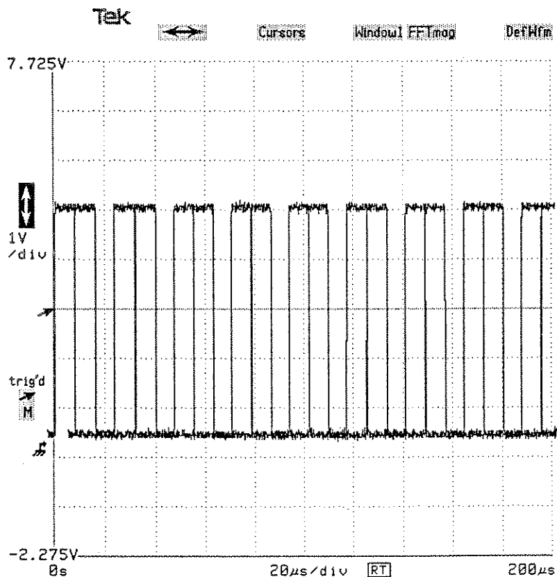
The Signal with Trigger Instability
