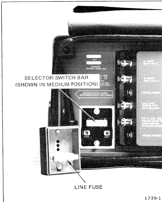
Fig. 1. Regulating range selector and line fuse.
