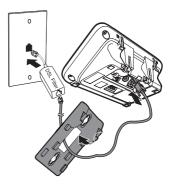
2 Align the holes on the bracket with the standard wall plate and slide the bracket down until it clicks securely in place.
