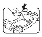
5. Pull up on metal rod to ensure legs are securely locked.
