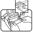
Pull the metal rod towards you, while the safety lock release buttons are being pressed. This will unlock the metal rod from the safety locks, allowing the legs to fold into the desired position.
