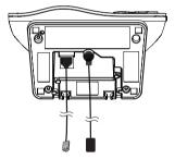
3. Position the lower portion grooves on the telephone base to the lower portion tabs (marked B) on the wall mount bracket. Make sure the upper portion grooves of the telephone base are above the upper portion tabs (marked A) on the wall mount bracket. Push the telephone base down until it clicks securely in place.
