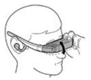
Vuzix' AccuTilt™ technology allows viewer adjustment through 15 degrees to properly align the viewer with your eyes. Grasp the viewer and tilt it until the displays are comfortably aligned with your line of sight. Each temple of the viewer pivots independently for precision adjustment.
